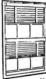
Shield to prevent light streak between sections
