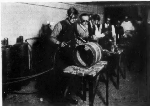
E VENING VOCATIONAL SCHOOL—A practical course in acetylene welding, a much-used process in modern industry.
